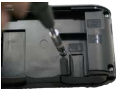
Image 9. Unscrew the battery holder. Image 10. Pull out the battery holder. Image 11. Loosen the cable and connect the new battery.
