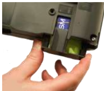
Image 9. Unscrew the battery holder. Image 10. Pull out the battery holder. Image 11. Loosen the cable and connect the new battery.
