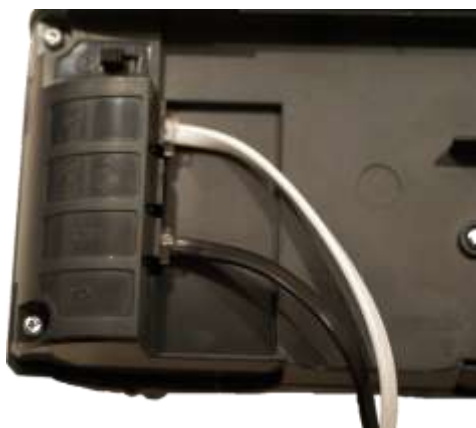
Image 3. Here you can see in which jack the telephone cable (white) and mains adaptor (black) are to be connected.
