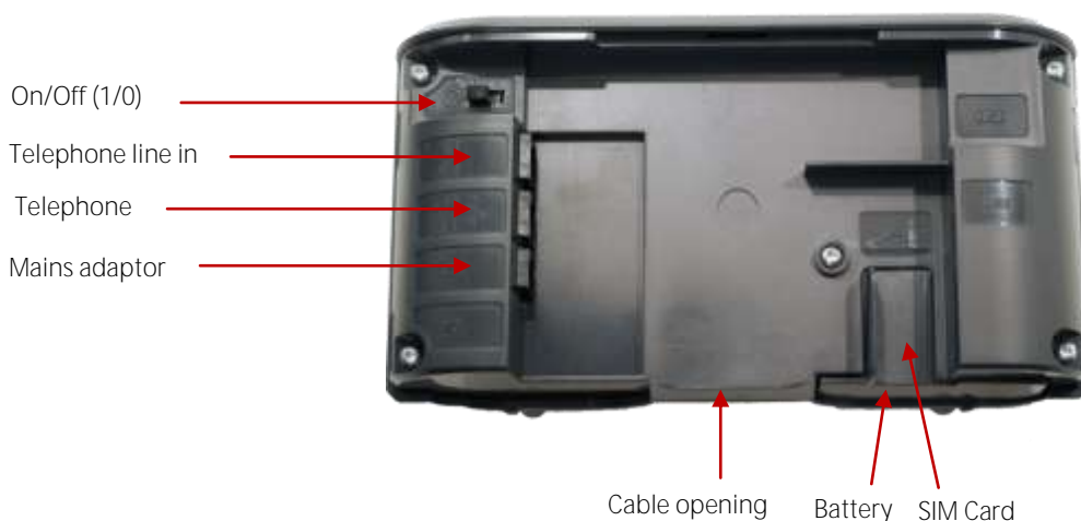
Image 2. Placement of connectors, battery and SIM card.
