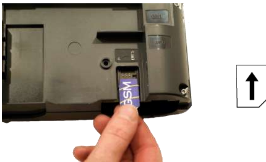
Image 4. Slide the SIM card into the SIM card holder.
