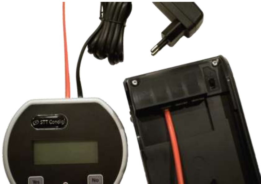
Image 8. Connect the red cable to the carephone and HT-III, and connect the mains adaptor to HT-III.
