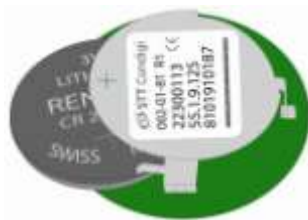
Image 16. Slide the new battery in. The plus side should be upwards.
