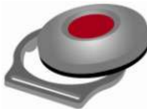
Image 19. Attach the ring by pressing it on from the back of the transmitter until a click sound is heard. Make sure the elevation on the inside of the ring fits to the notch of the plastic bottom part of the transmitter.
