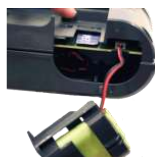
Image 9. Unscrew the battery holder. Image 10. Pull out the battery holder. Image 11. Loosen the cable and connect the new battery.
