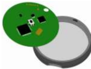
Image 17. Place the circuit board in the new plastic bottom part. Make sure the hole at the edge of the circuit board is placed over the elevation at the edge of the plastic bottom part.
