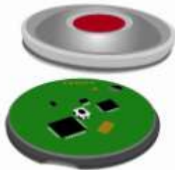
Image 18. Turn the new silicon cover inside out and place it against the circuit board before you turn it back.
